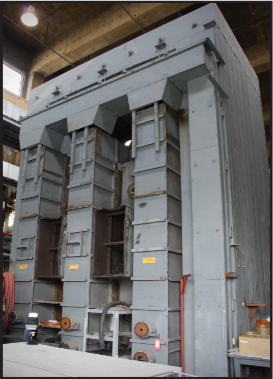
World's only Alpha Calutron magnets (Courtesy of Y-12 National Security Complex)
