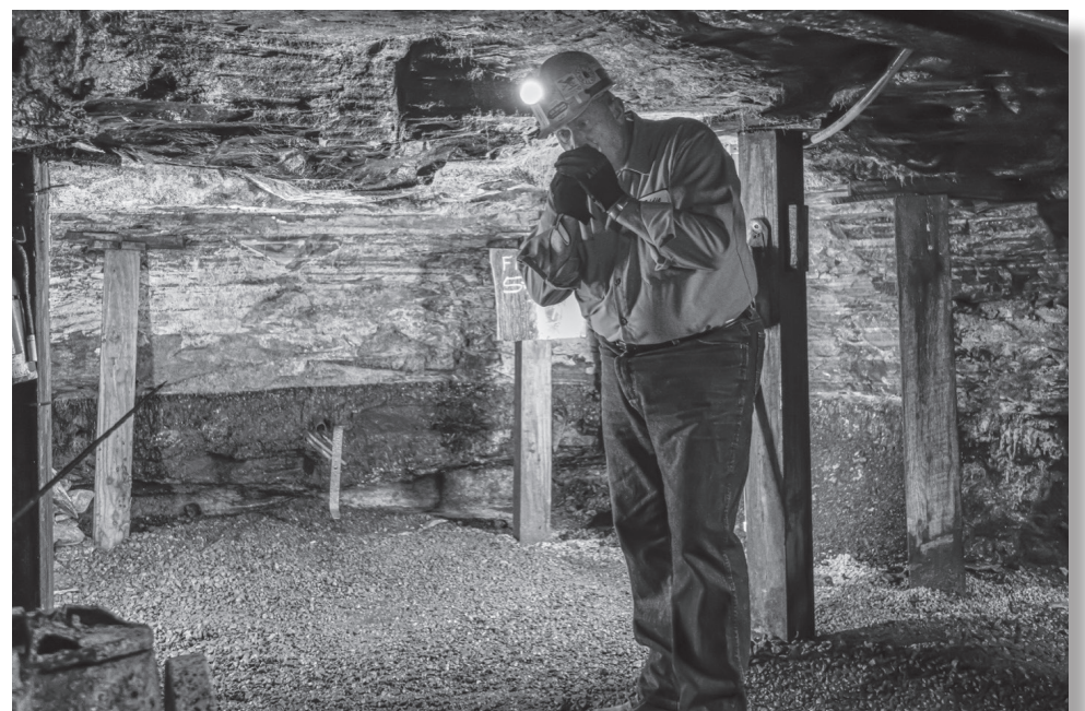
A view of the 18-24 inch coal seam in the Beckley Exhibition Coal Mine. Miner’s previously were not paid for removal of the rock above the seam to provide headroom. [Photo by Terry Futrell]
